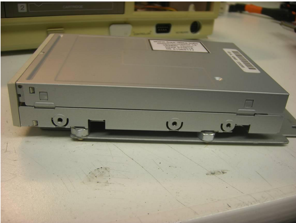
The new disk drive with spacers on the bottom plate.
